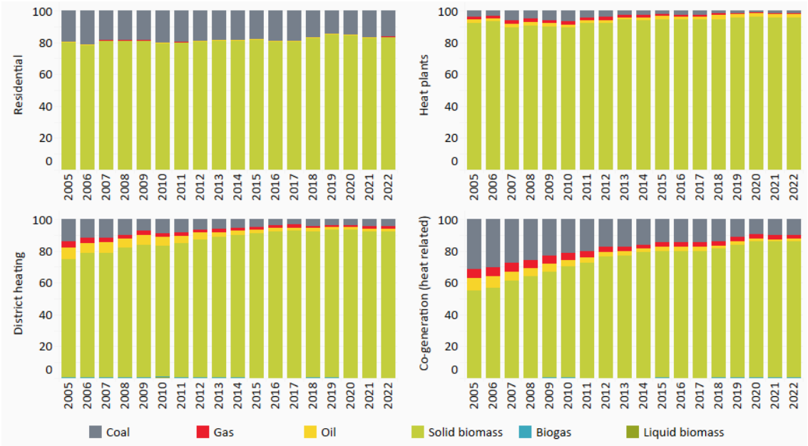
Figure 22. Contribution of fuels to PM 2.5 emissions from heat-related activities in the EU-27, 2005–2022 (%)
