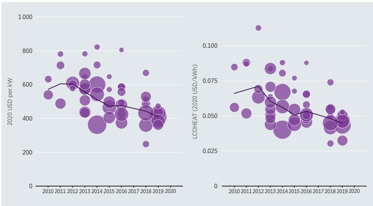
Figure 9.1 Total installed costs and LCOHEAT for solar thermal district heating plants in Denmark, 2010-2019
