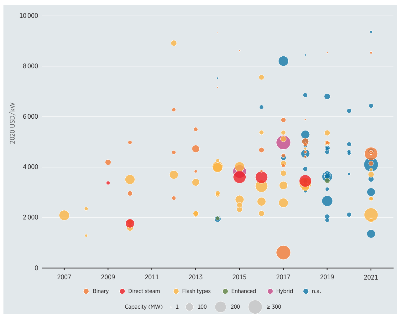
Figure 7.2 Geothermal power total installed costs by project, technology and capacity, 2007-2021
