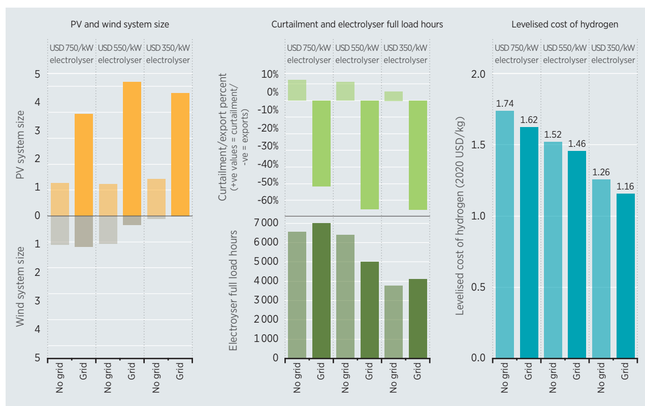
Figure 1.11 Scenarios for LCOH 2 from utility-scale solar PV and onshore wind under different input assumptions in Saudi Arabia
