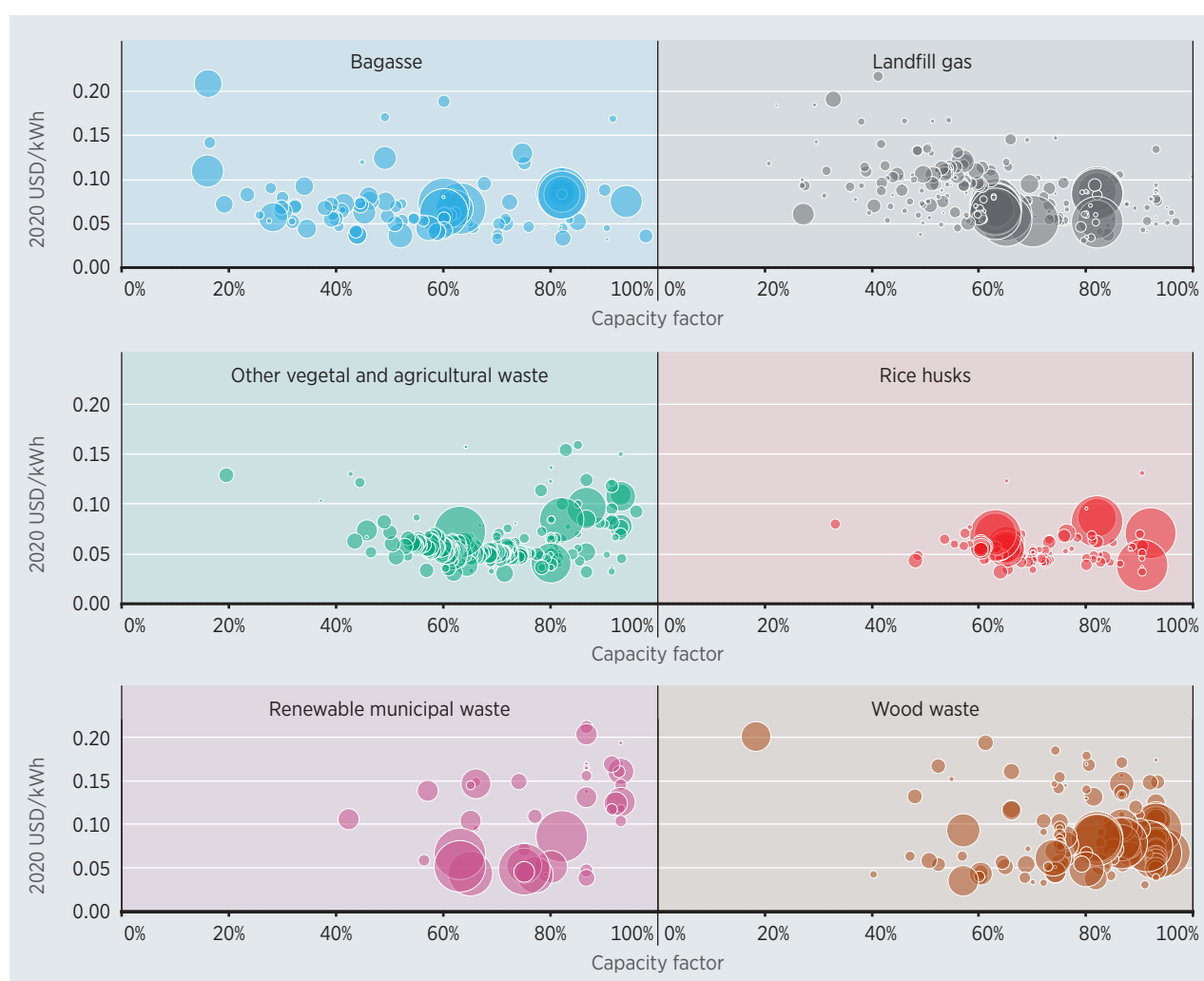
Figure 8.6 LCOE and capacity factor by project of selected feedstocks for bioenergy power generation projects, 2010-2020
