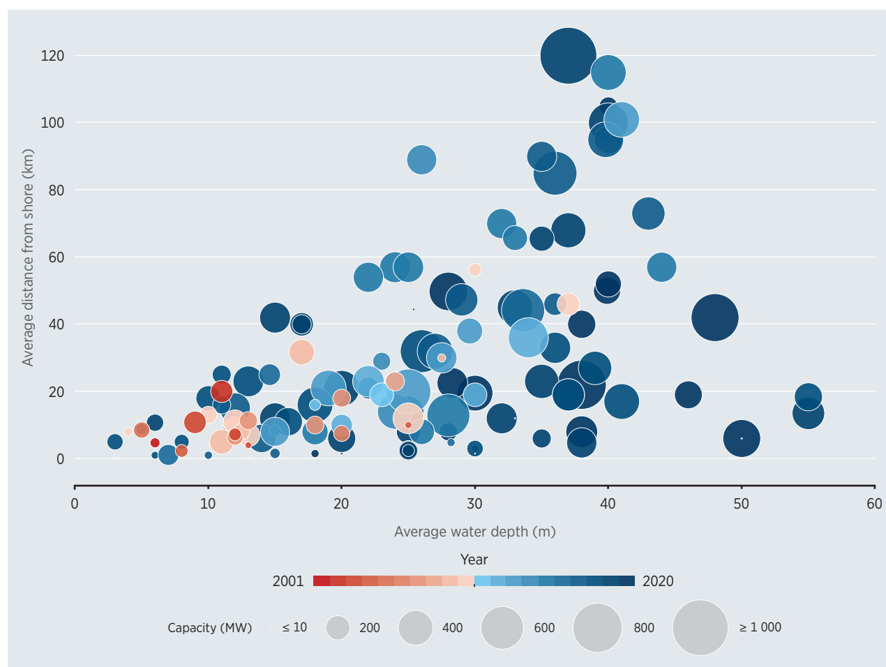
Figure 4.2 Average distance from shore and water depth for offshore wind, 2000-2020
