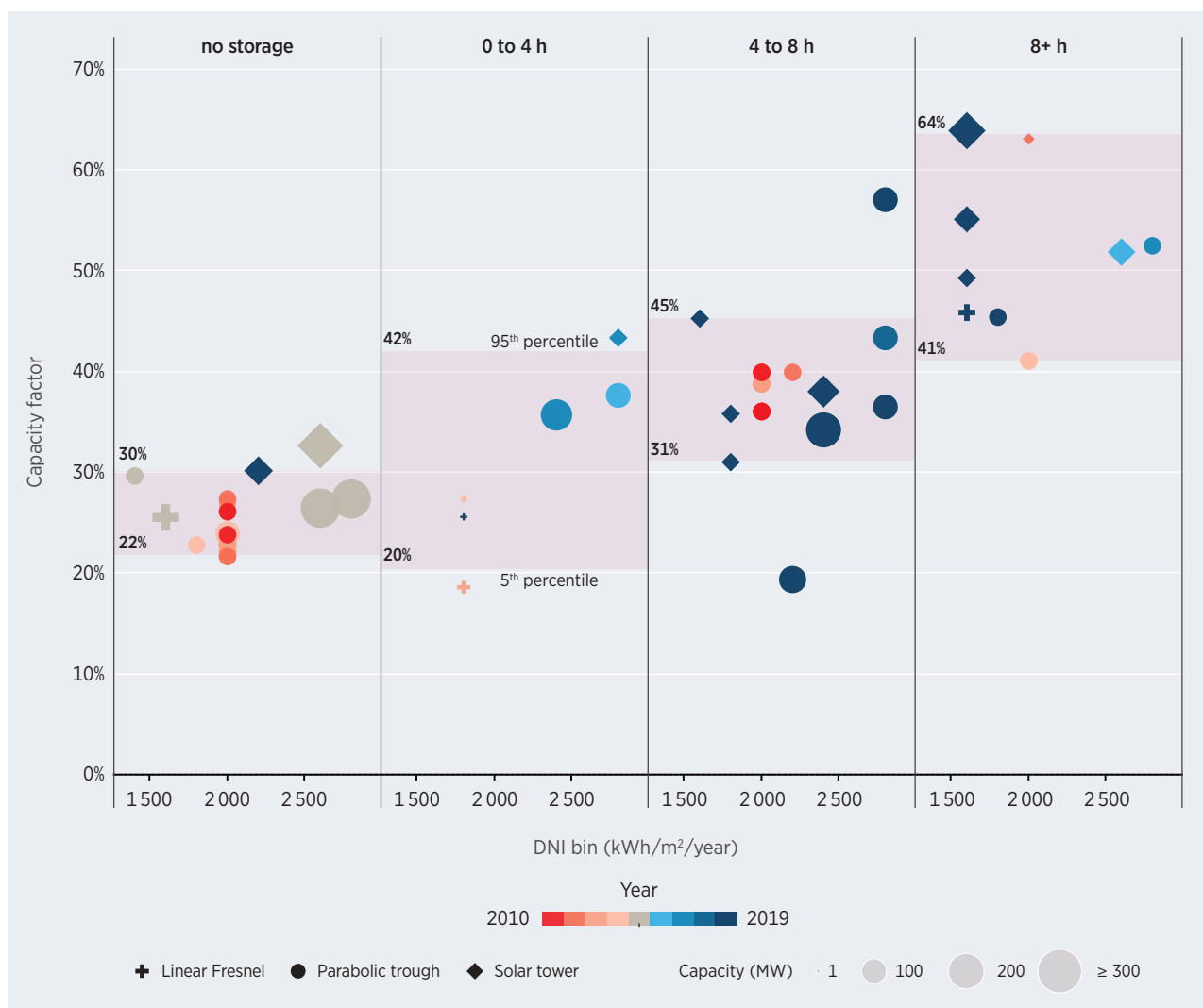
Figure 8.4 Capacity factor trends for CSP plants by direct normal irradiance, 2010-2019
