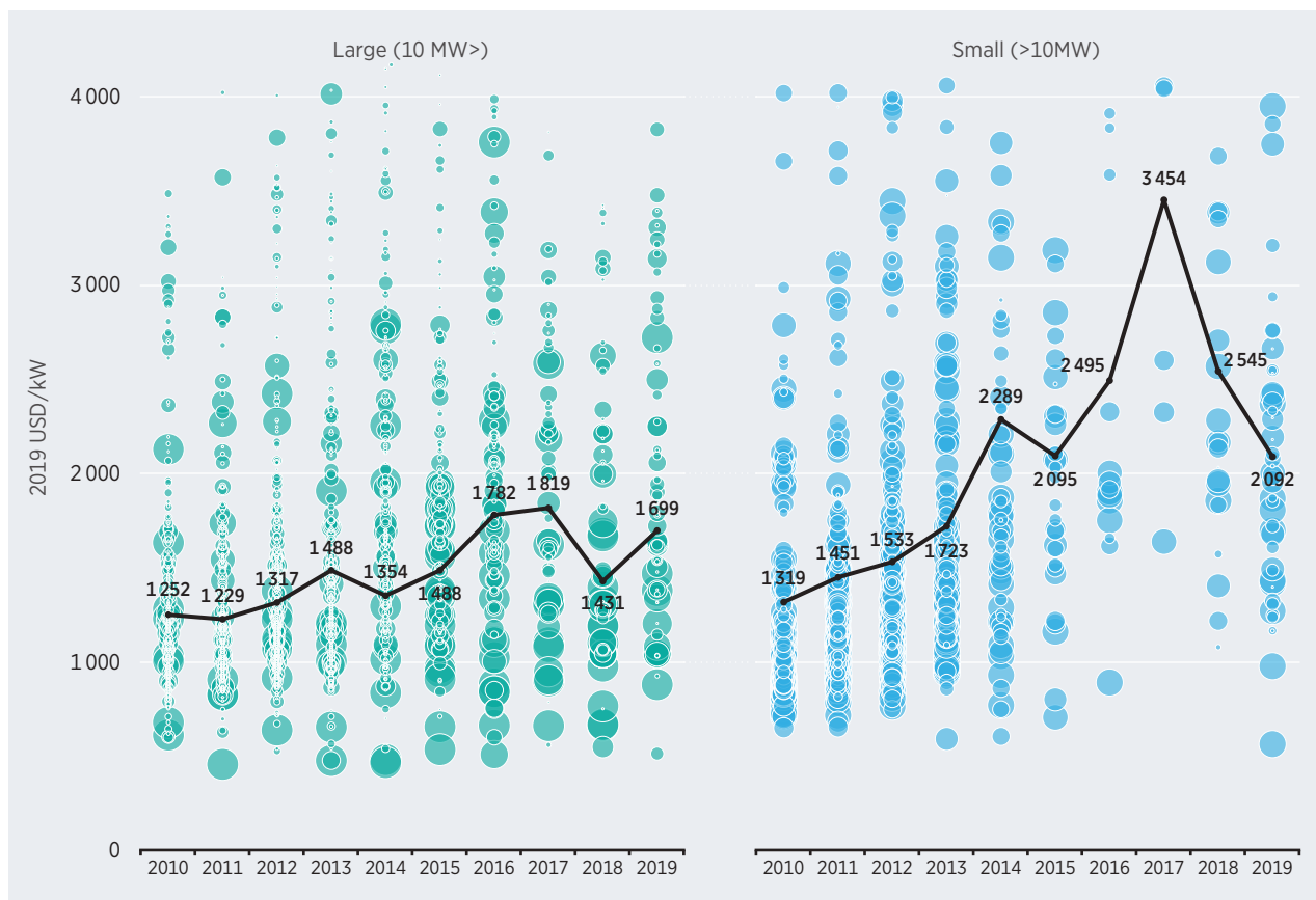
Figure 5.3 Total installed costs for small and large hydropower projects and the global weighted average, 2010-2019
