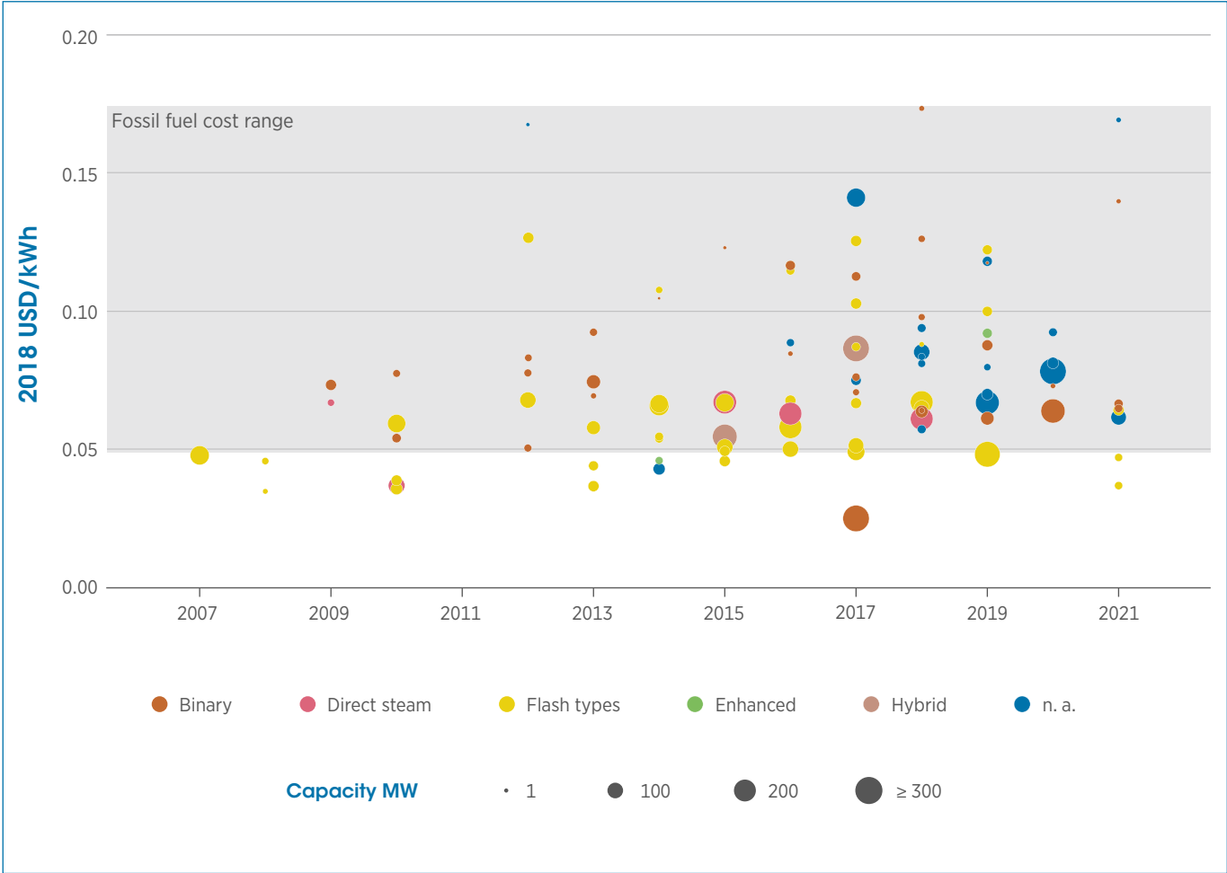
Figure 6.3 LCOE of geothermal power projects by technology and size, 2007–2021
